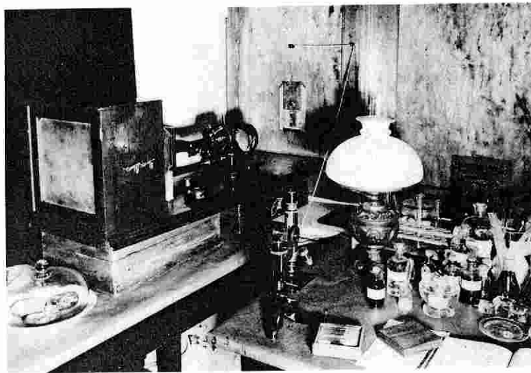
Figure 7.3 Reconstruction of Robert Koch's work room in Wollstein, as shown at a Robert Koch exhibition in Berlin in 1935. The horizontal photomicroscopic apparatus Koch used in his later work is on the left. Note the string-operated shutter that controls the admission of sunlight into the room.
