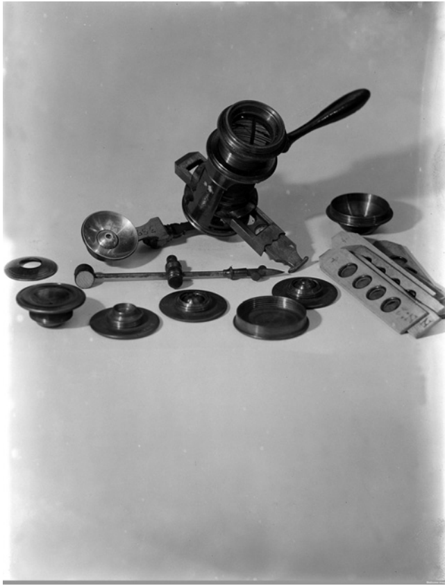
Figure 36.2 A screw-barrel microscope made to James Wilson’s design, with a variety of lenses and slides. Wellcome Library, London.
