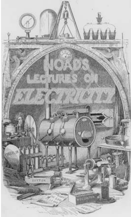
3.3 The frontispiece of Henry M. Noad's Lectures on Electricity (1844) showing an idealized (if messy) electrician's workshop. In the foreground is an Armstrong hydro-electric machine, and a Wheatstone and Cooke five-needle telegraph hangs on the wall behind it. Various items of electricians' apparatus such as induction coils and batteries are scattered around. On the right, on top of the arch, is Grove's gas battery, illustrating the correlation of physical forces.
