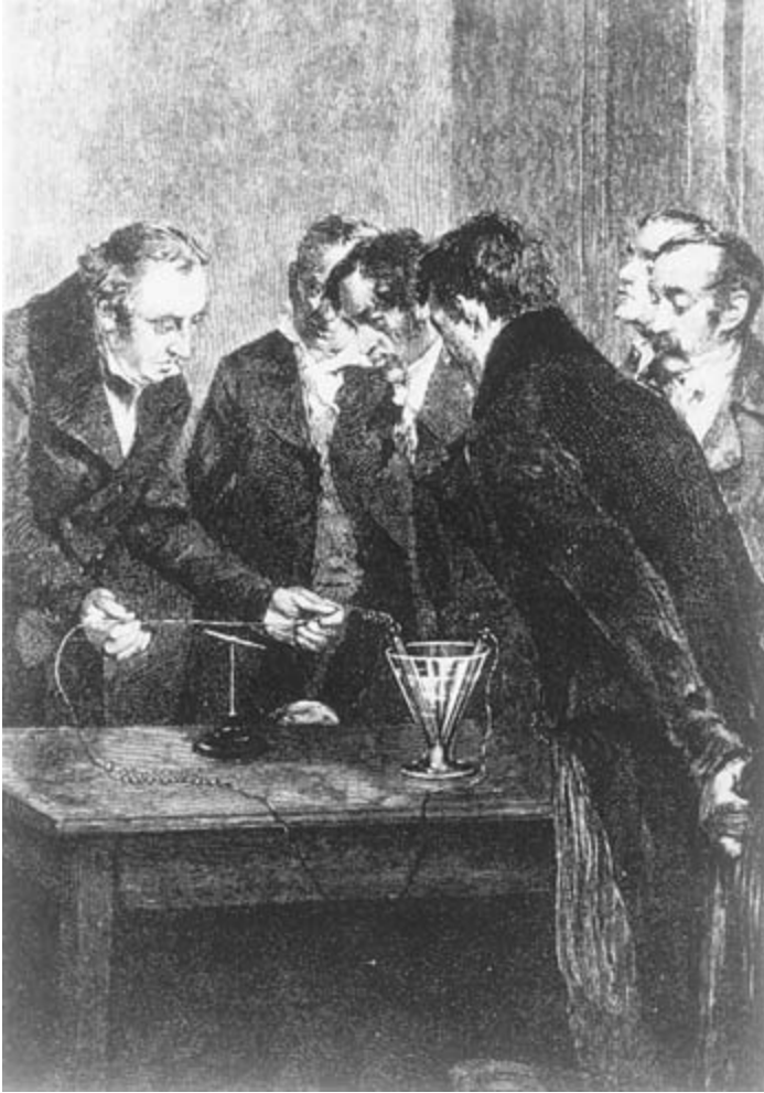
3.2 A nineteenth-century artist's impression of Hans Christian Oersted's 1820 observation that a magnetized needle held near a wire carrying a current of electricity was deflected.
