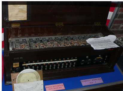
An American machine for decrypting the Japanese code, named PURPLE.
