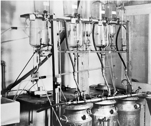
Ernst Chain's penicillin production setup
