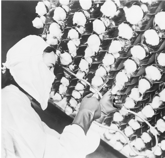
Growing the penicillin mold in individual flasks
